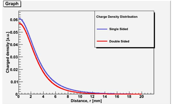
Fig 4. Charge Density Distribution for both TRD geometries – single-sided and double-sided.
