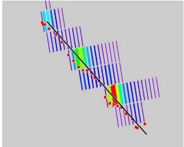
Fig. 4 the Tracklet is rendered as a linear fit of the clusters.
