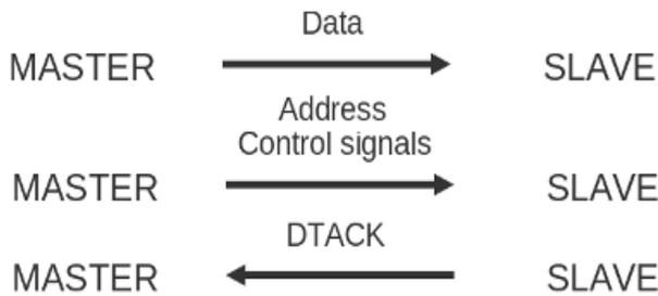
Fig 3 Handshaking protocol diagram
