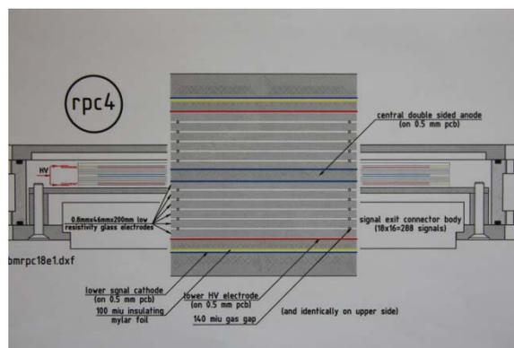
Fig 7 The assembly - graphic made - and a pop-upped section
