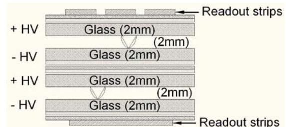
Fig 2 Schematic of a double gap Resistive Plate Chamber<sup>[4]</sup>
