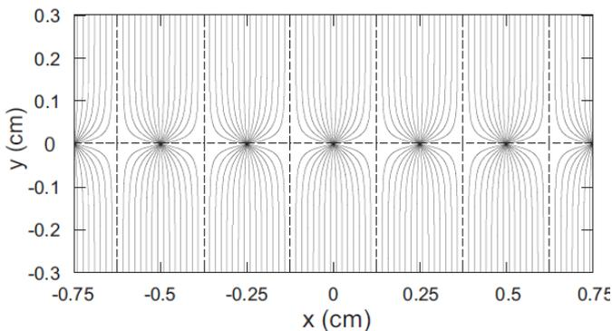
Fig 1. Schematic view of the electric field in an MWPC.
