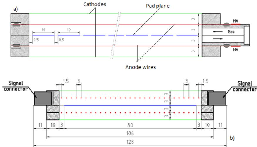
Fig 2 Schematic configuration of the TRD prototype: a) projection on a plane perpendicular to the detector surface and parallel to the wire direction and b) projection on a plane perpendicular to the detector surface and anode wire plane.
