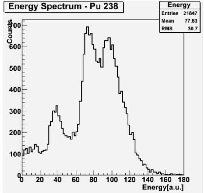
Fig 5. Energy Spectrum for <sup>238</sup>Pu.
