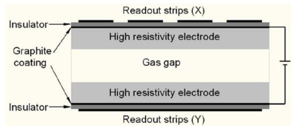
Fig 1 Constructional schematic of the original Resistive Plate Chamber
