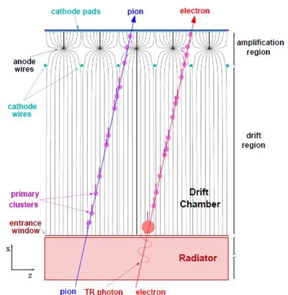
Fig 3 The cross-section through the detector, parallel to the direction of the anode wires for ALICE - TRD.
