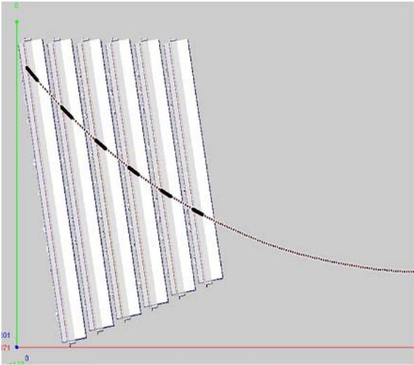
Fig. 2 TRD detector stack, simulated MC track and the detector "hits"
