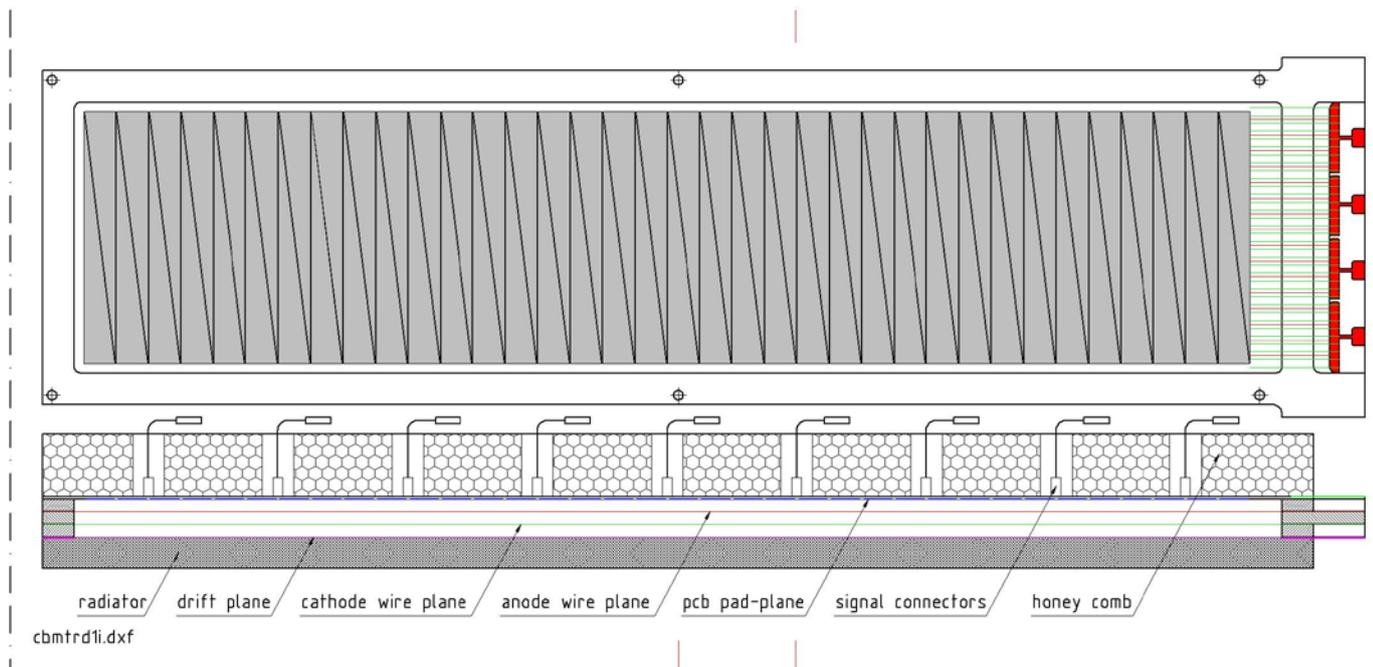
Fig 2. The pad plane design and the cross-section through the detector - perpendicular to the direction of the anode wires.
