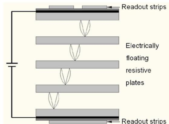
Fig 3 Schematic of a multi-gap Resistive Plate Chamber<sup>[9]</sup>
